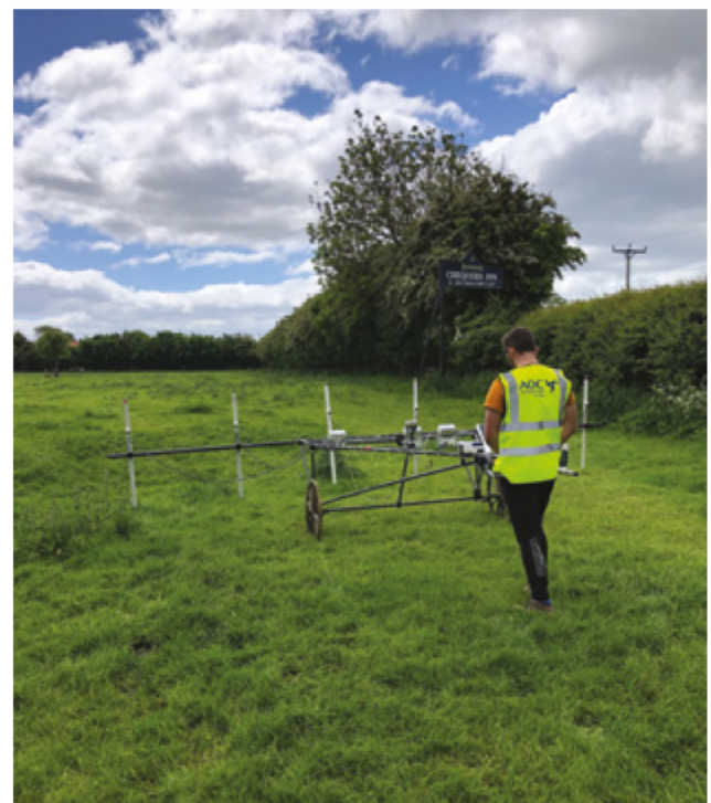
A gradiometer fitted to a hand-pushed cart used during archaeological surveys.
